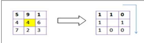
Figure 2. The basic Local Binary Pattern Operator (LBP)
