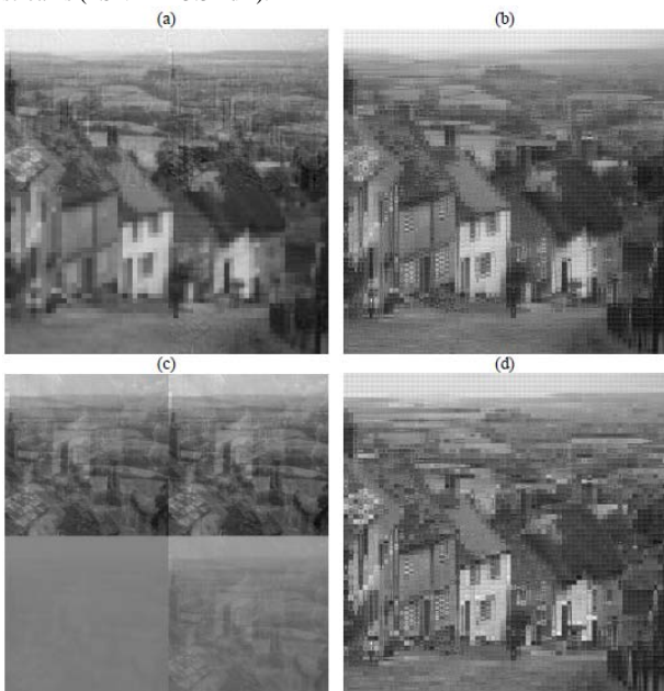
Fig. 11. Goldhill image reconstruction results with three packets lost, at 2 bits/sample. (a) MDTC_TEC1 with DC coefficients communicated reliably with some other means (PSNR = 24.74 dB); (b) MDTC_TEC2 with DC coefficients communicated reliably with some other means (PSNR = 23.88 dB); (c) MDTC_TEC1 with DC coefficients communicated with the four data streams (PSNR = 16.13 dB); (d) MDTC_TEC2 with DC coefficients communicated with the four data streams (PSNR = 21.32 dB).
