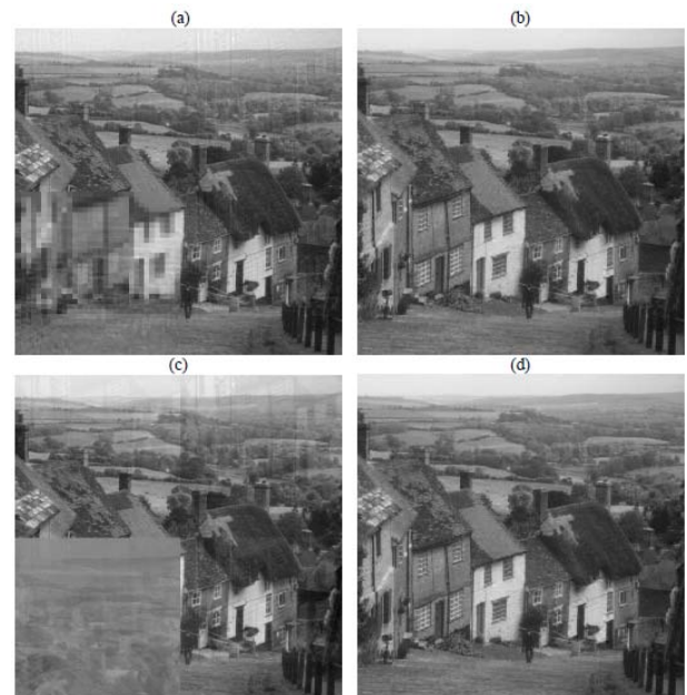
Fig. 9. Goldhill image reconstruction results with one packet lost, at 2 bits/sample. (a) MDTC_TEC1 with DC coefficients communicated reliably with some other means (PSNR = 28.03 dB); (b) MDTC_TEC2 with DC coefficients communicated reliably with some other means (PSNR = 33.68 dB); (c) MDTC_TEC1 with DC coefficients communicated with the four data streams (PSNR = 22.12 dB); (d) MDTC_TEC2 with DC coefficients communicated with the four data streams (PSNR = 33.60 dB).
