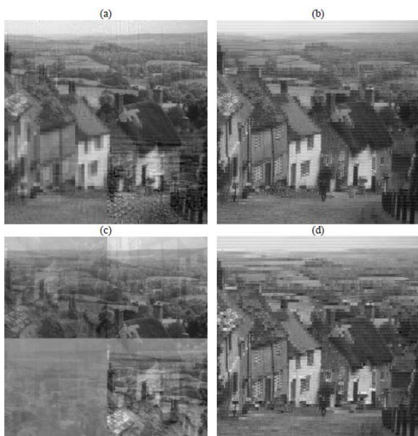
Fig. 10. Goldhill image reconstruction results with two packets lost, at 2 bits/sample. (a) MDTC_TEC1 with DC coefficients communicated reliably with some other means (PSNR = 25.45 dB); (b) MDTC_TEC2 with DC coefficients communicated reliably with some other means (PSNR = 26.31 dB); (c) MDTC_TEC1 with DC coefficients communicated with the four data streams (PSNR = 17.24 dB); (d) MDTC_TEC2 with DC coefficients communicated with the four data streams (PSNR = 23.32 dB).
