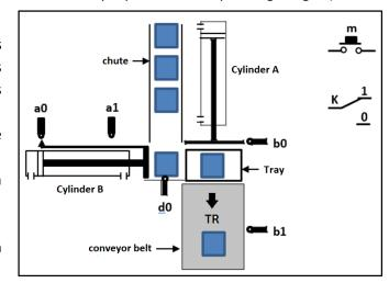
Once the rod of cylinder B returns to position **b0** and the 4-second duration has elapsed, the next cycle can begin.
