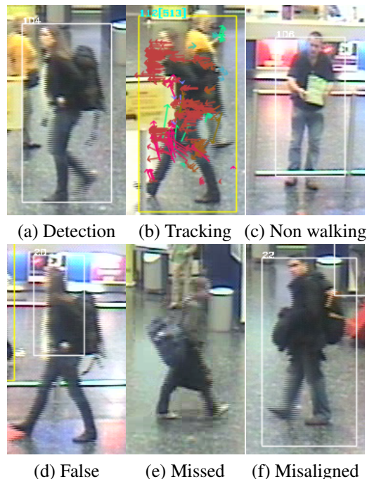
Figure 1. HoG based person detection results. Positive detection of a walking (a) and non walking human (c). Expected errors are false, missed and misaligned detections (d-f). In case of partial occlusions (b), detections are tracked using feature point motion (color coded arrows).
